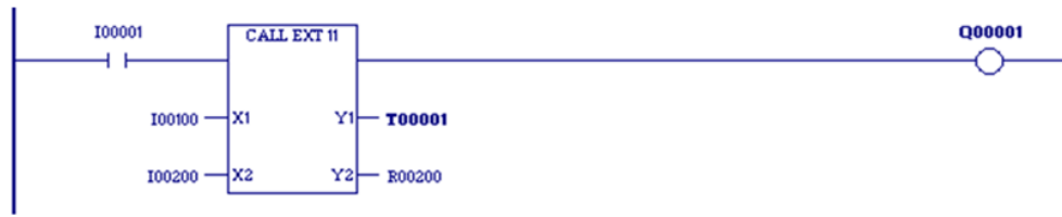
Figure 8: Calling an External Block in Ladder Logic
