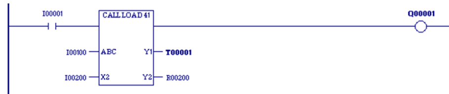
Figure 3 Block Call with Parameters
